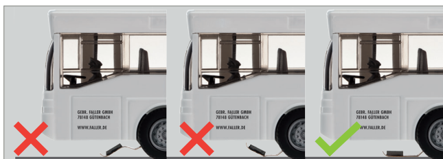
Fig. 3: Adjustment of the steering rod
